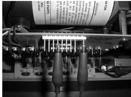
If the original Swell Shoe Simulator Switch is no longer available when you begin to set up your re-installed Peterson Model C Swell Shade Operator, you can simply use a clip lead to connect the Positive Common pin to each expression contact input pin, in turn, as shown in these photos.
